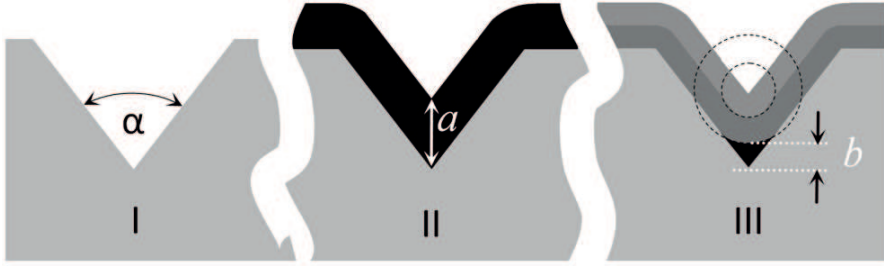
Figure 3.1: Corner Lithography concept (cross-sectional view): (I) V-groove template preparation, angle \alpha , (II) deposition of conformal material, layer thickness t and thickness a in the corner, and (III) time controlled selective isotropic thinning by distance r leaving a nano feature of height b .
